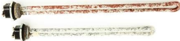
Water heater makes less hot water because calcium is building up on heating elements and reducing heat transfer efficiency
